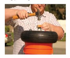
\*Please note that Austin uses a screwdriver to remove the bearings/bushings because that is a common household tool. Screwdrivers are not intended as "striking" tools and a steel rod or other strong metal rod may be more effective. Use a screwdriver at your own risk.
